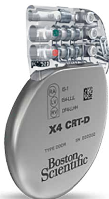
Boston Scientific's implantable cardiac resynchronization pacing & defibrillator device.
